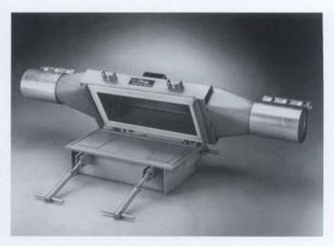
Dings' design has a plate magnet that swings away for easy and safe external cleaning, which protects against accidental "wipe-off" of tramp iron into the line. To clean the plate, simply loosen the clamping handles and swing the magnet open. Then wipe any tramp metal off the plate magnet. And, since the Dings' surface area is 37% larger than competitive designs, it holds more tramp metal — enabling you to wait longer between cleanings.
